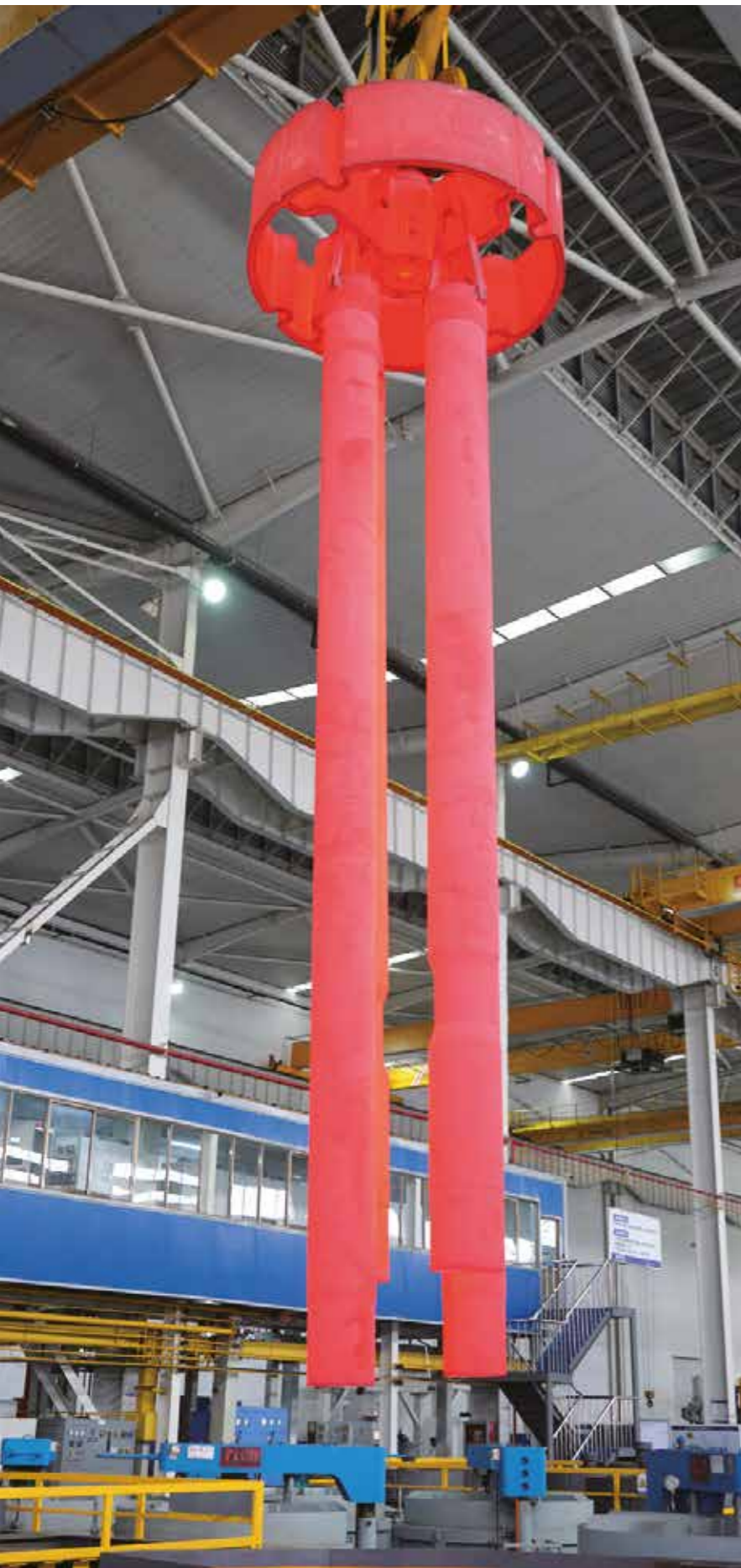
Example of in-house tie bar manufacturing with efficient FMS lines (above) and immersion basins (left)
