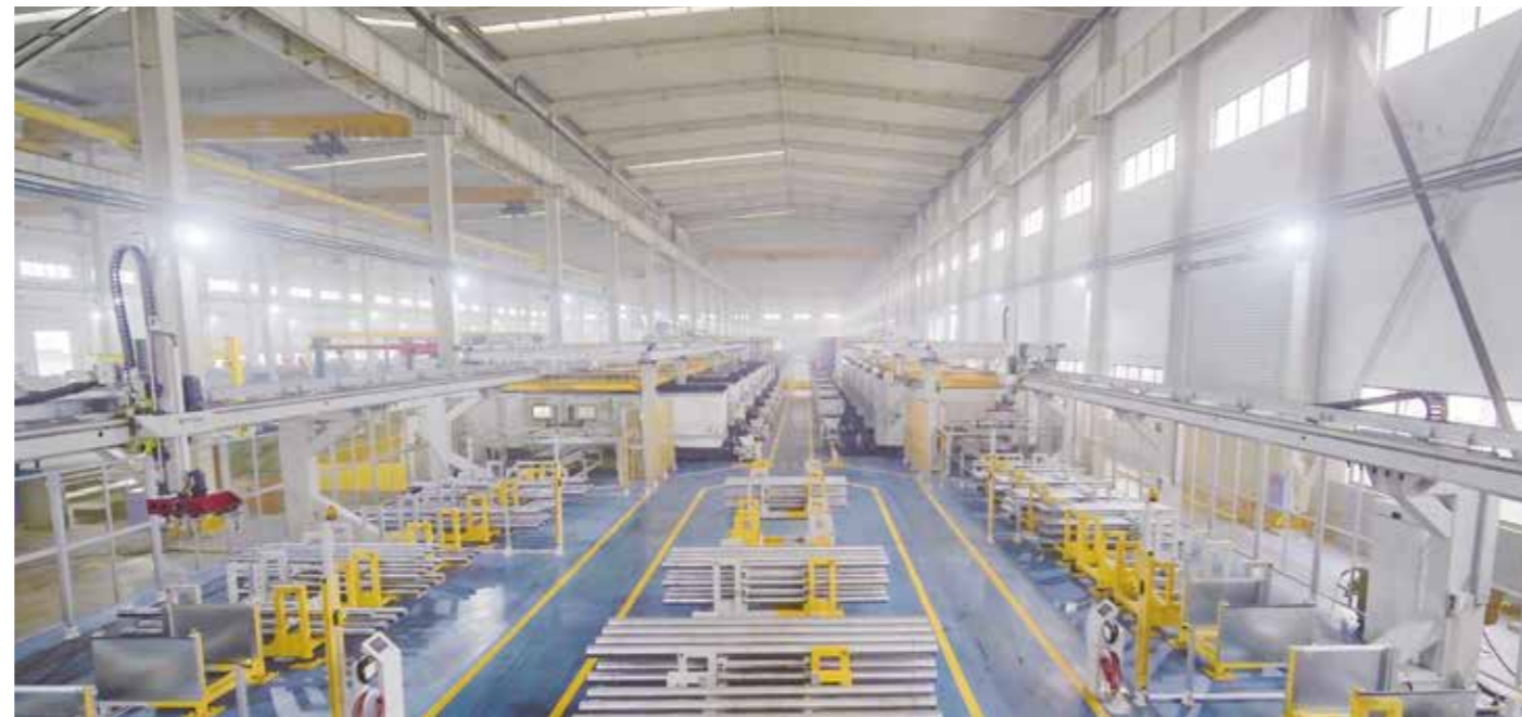
Example of in-house tie bar manufacturing with efficient FMS lines (above) and immersion basins (left)
